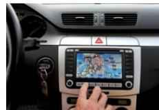
it is from each satellite's position and distance. Usually there must be at least four satellites to solve the geometric equations. A GPS receiver can calculate its position many times in one second.
